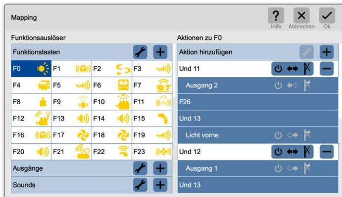
Representation of a complex mapping. The information is spread over two pages. The function activates "And 11". "And 11" activates "Output 2" and "Front light". "Front light" in turn has the other triggers F26 and "And 13". F26 and "And 13" are new in this display and extend the understanding of when an action is triggered. It is now possible to see when and how these triggers work. The trigger conditions are only shown in the direct trigger chain.
