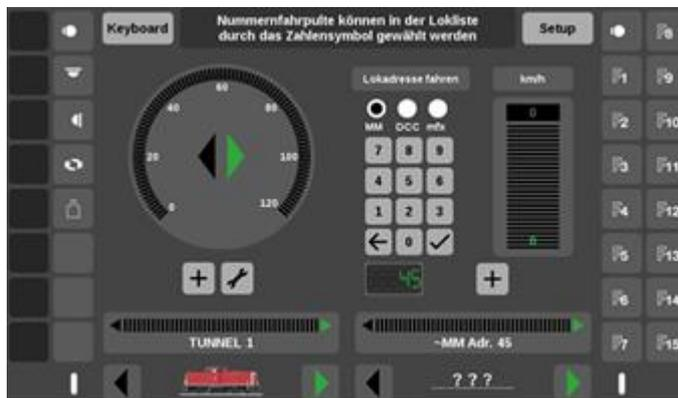
The situation is similar for a receiver to switch turnouts. Directly implemented is a user interface for up to 32 double coil solenoid turnouts. Via the "keyboard" button you get to this control panel. Simply set the receiver to one of these associated addresses (1 to 32), connect the receiver to the layout track output or programming track output of the CS 3 and you can test it.
